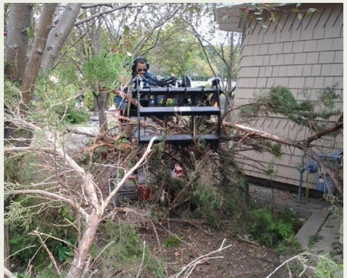
Ryan Sullivan, the park keeper at Lake Harriet, used the grapple rake to remove large junipers from this very narrow space without damaging the building or utilities.
