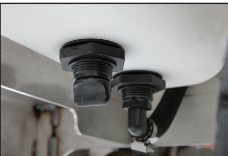
Drain plug at the lowest part of the tank allows for quick and convenient tank draining and cleaning in between the use of different chemicals.
