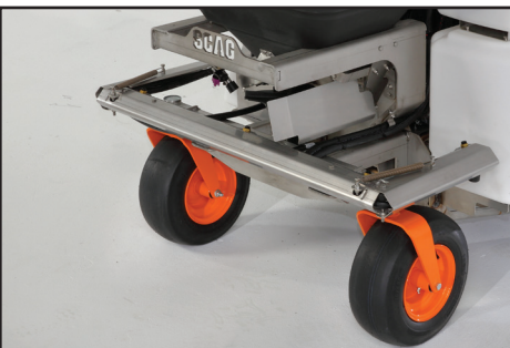
Hinged boom arms fold inward for transport, or to access tighter spaces.
